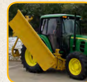
Inboard and Outboard adjustment controlled by hydraulics.
