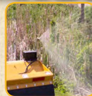
Offset Sprayer can reach weeds up to 14 feet from the right of the mower deck.
