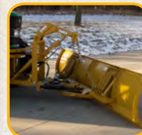
Dual Cylinders built for Angling Plow.
