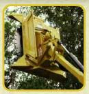
**SAW BLADE** 48" saw blade diameter
