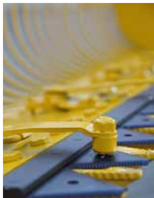
Cutter bar with spring pressure holder for continuous knife pressure.
