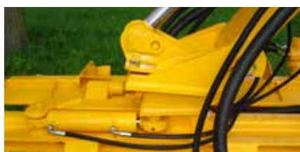
Hydraulic 90° rotating head by means of a cylinder (HD90).
