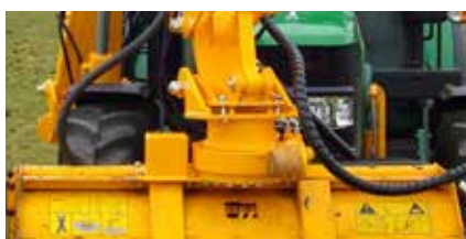
Hydraulic 180° rotating head by means of a worm gear turntable (HW180).
