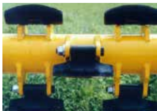
Heavy-duty wood flail (2.3 kg). It is ideal for mowing wild shoots and woody vegetation.
