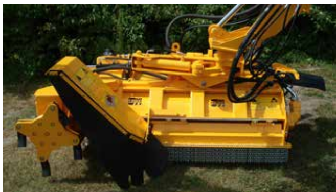
Bottom fraise unit for mowing the bottom of the ditch and the slope in one run.
