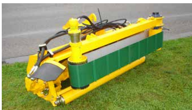
Conveyor belt unit in the heavy-duty model for grass removal when mowing ditches and slopes.
