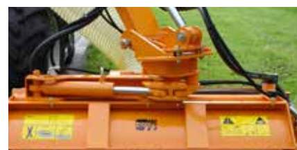
Hydraulic 180° rotating head by means of a cylinder (HD180).
