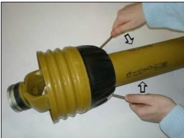
Pry clasps open to release the shield
