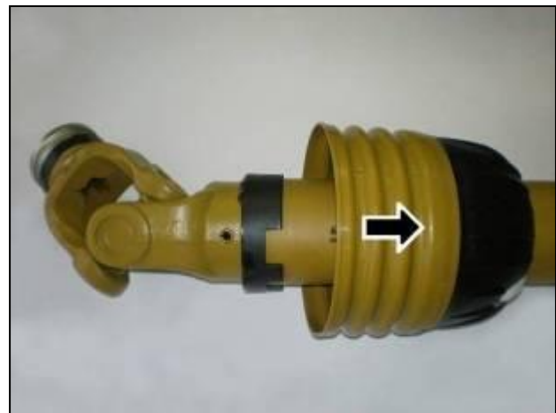
Slide shield back to reveal universal joint
