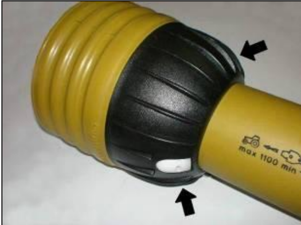
Shaft shield fixing clasps
