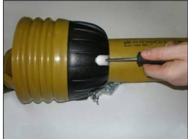
Insert screwdrivers into the clasps
