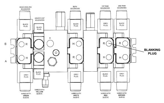
WIRING DMV VALVE - 4 SERVICE
