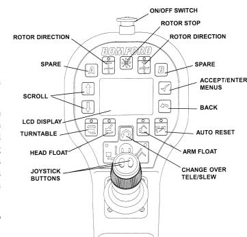
Slew and Telescopic Arm Operation – Both operations are controlled by the joystick buttons. Depress the change over button to select the function required which will be indicated by an LED (light emitting diode) indicator.
