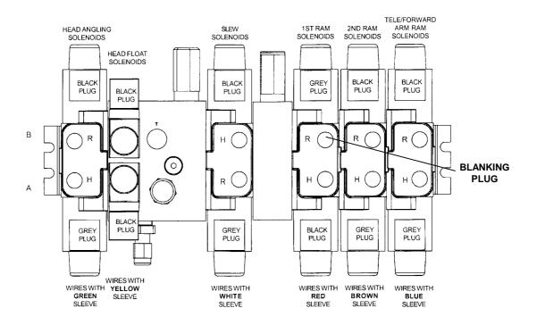
WIRING DMV VALVE - 5 SERVICE
