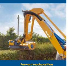
Enables mid-mounted head position with simplicity of rear
