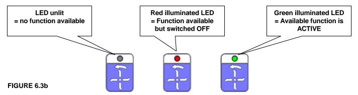
Each button is accompanied by a bi-colour LED. When the control box is connected and powered up all available services are illuminated in red. LED's which remain 'off' indicate services which are not available on the machine. When a red illuminated (available) LED service is subsequently activated the LED changes colour from red to green.
