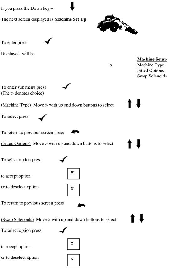
With this facility it allows operations of functions to be swapped without changing the wiring or hoses
