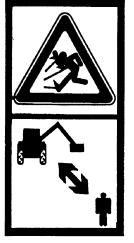
DANGER FROM THROWN DEBRIS. KEEP ALL PERSONNEL AT A SAFE DISTANCE FROM THE MACHINE WHEN WORKING
