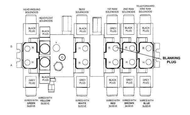
WIRING DMV VALVE - 5 SERVICE
