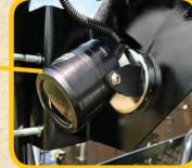
Optional camera located on the right side of the TrucKat allows the operator to view the cutting head in operation while facing forward and steering vehicle.
