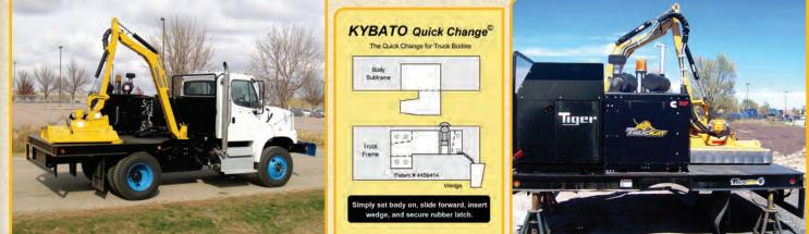
Remove the Tiger TrucKat in minutes with the use of the patented Kybato Quick Change system. The quick disconnect system allows the truck to be used for other applications throughout the year.
